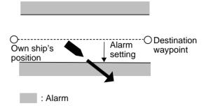
Figure 8-7 How the XTE alarm works
